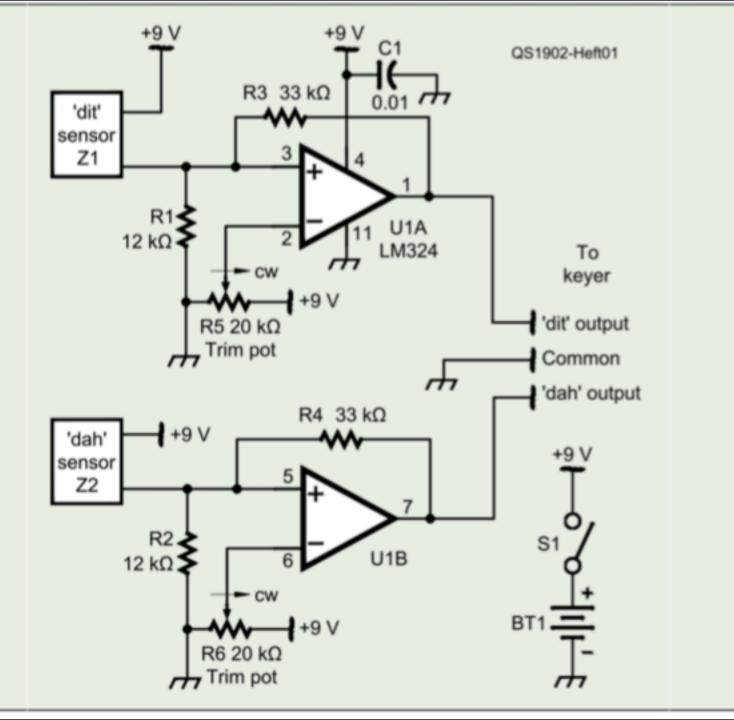
QST February 2019 A Force-Sensing CW Paddle Art Heft, K8CIT Errata: Pins 2 and 3 of U1A and pins 5 and 6 of U1B should be swapped
