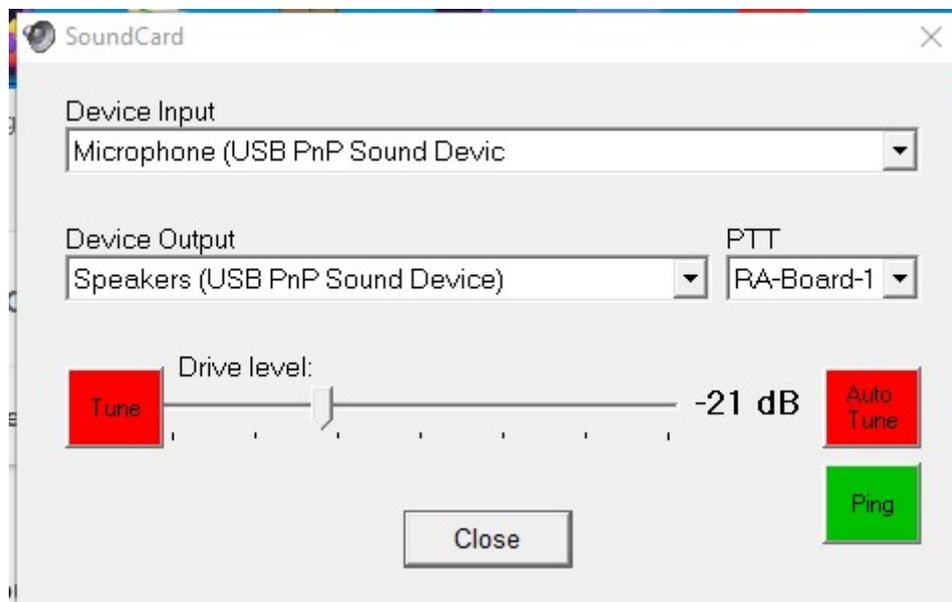
The Autotune adjust automatically the Drive Level but, also, will show a warning message if any level is not right (useful for new users):
