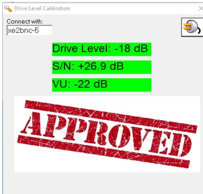
The Ping function show the viability on both directions, either connecting directly, or using digipeaters. In case of digipeaters, the S/N value is the minium along the chain. So, using diferent digipeaters you will have better or worse S/N to reach a same station. The VU levels is useful for monitoring if any station is saturating or has a weak audio input level (below -40dB):
